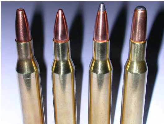
.270 ammunition, L to R: 100-grain (6.5 g) – hollow point 115-grain (7.5 g) – FMJBT 130-grain (8.5 g) – soft point 150-grain (9.7 g) – round nose (Full Metal Jacket Boat-Tail)
