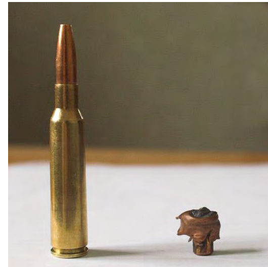
6.5x55mm ammunition, before and after expansion
